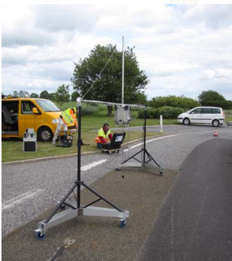
Sound absorption measurement of PERS in Arnakke. Round robin tests between Ifsttar and DRD in June 2012
