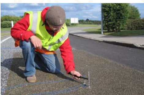
Mechanical impedance testing of PERS by Ifsttar in Arnakke in June 2012
